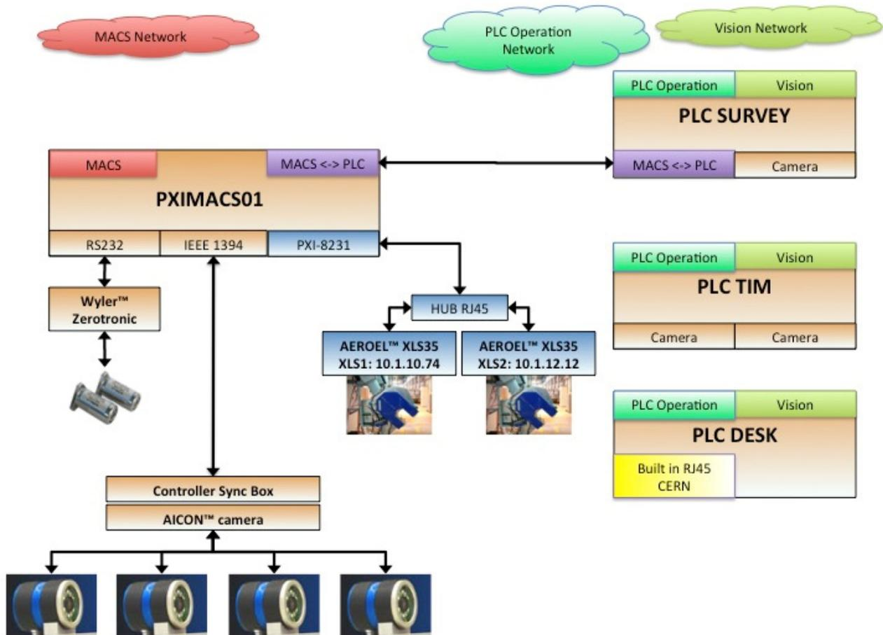
Figure 3: Instrumentation and communication layout of TIM and MACS.
