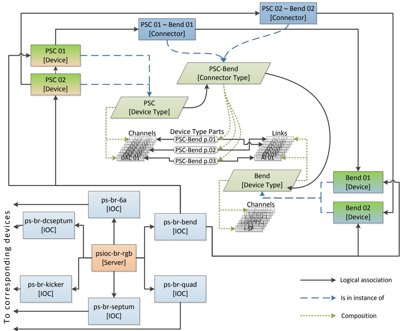
Figure 2: Simplified part of configuration information graph for NSLS-II Booster magnetic subsystem.
