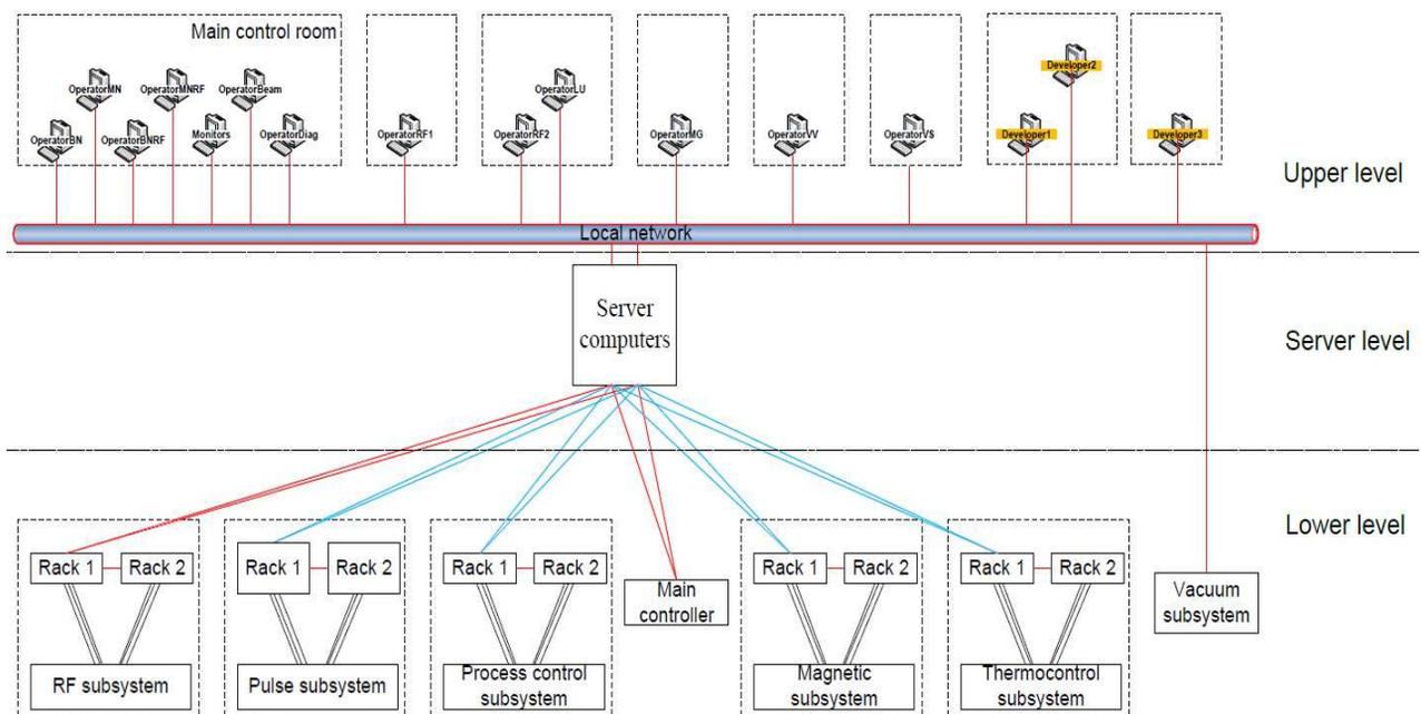
Figure 1: The layout of new automated control system at Kurchatov synchrotron radiation source.
