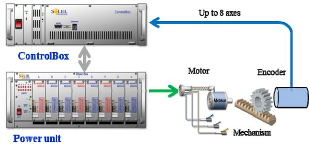
Figure 1: Standardized hardware architecture.
