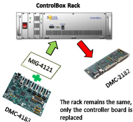
Figure 4: Replacement of controller into CONTROLBOX.
