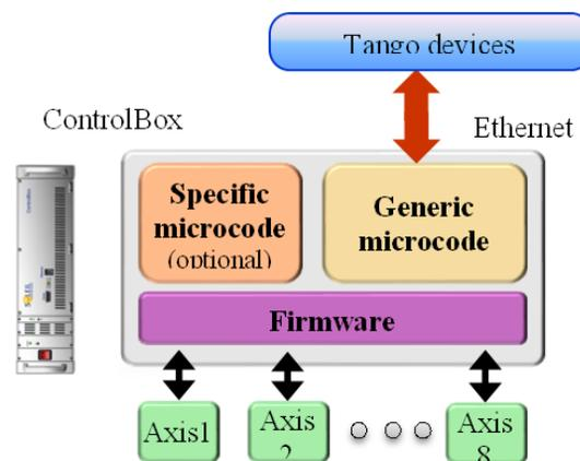
Figure 2: Microcode and Tango devices.
