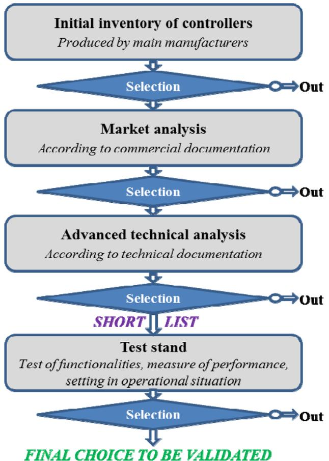
Figure 5: High performance controller selection steps.
