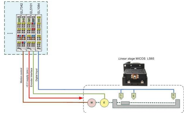
Figure 3: General motor electronic control.
