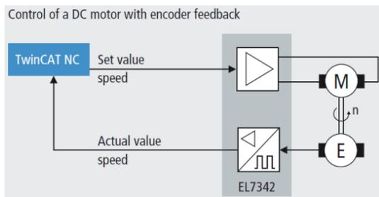
Figure 2: Beckhoff TwinCAT NC axis velocity control loop.
