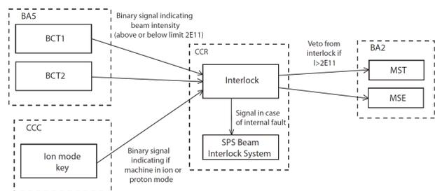
Figure 2: Schematic of the principle of protection.
