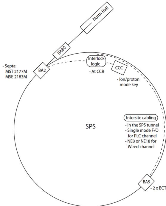
Figure 3: The geographical layout of the safety system components within the SPS ring.
