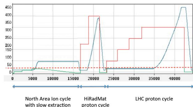
Figure 1: A typical SPS super cycle during a primary ion mode run, comprising an SFTION at 80 GeV/c/charge, a HiRadMat at 400 GeV/c and an LHC cycle at 450 GeV/c. The blue line represents the magnetic rigidity, the green line (red above the  $2 \times 10^{11}$  threshold) the number of charges. The threshold level (dotted line) is exaggerated for the drawing to be readable. The momentum scale is in GeV/c/charge, the time scale is in ms.
