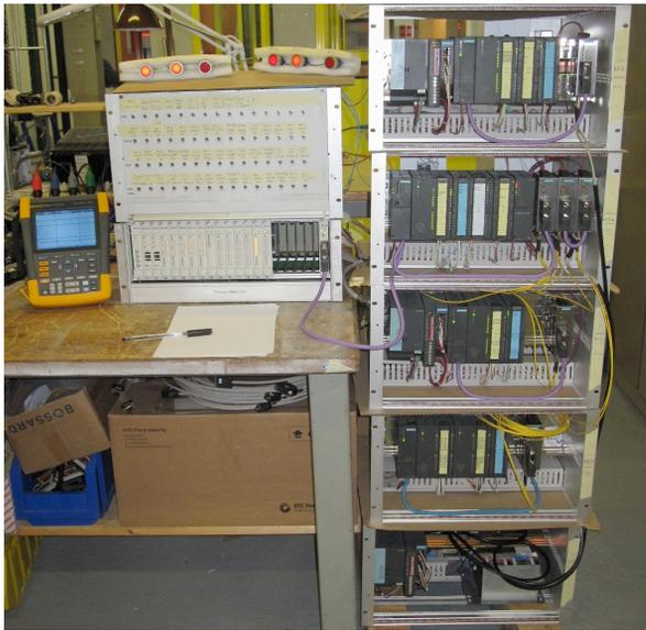
Figure 5: The wired and PLC interlocks in the test bench. The HIMA rack is on the left hand side at the bottom and a switch matrix to simulate different signals at the top. The PLC rack with remote I/Os in separate sub-racks is seen on the right.
