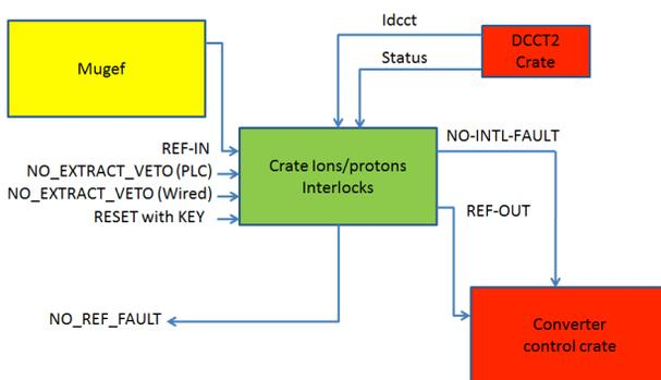
Figure 6: Power converter signal diagram. The reference is sent as an analog signal directly from the SPS power converter control system (Mugef). Interlock signals from both PLC and wired channels are shown as well as the internal safety-check signals from the special DCCT installed.
