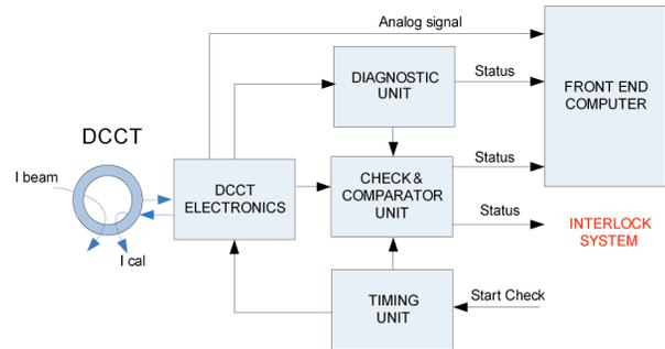
Figure 4: Block diagram of the BCT subsystem.
