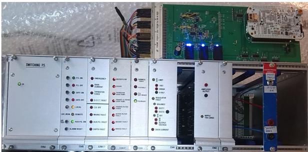
Figure 7: Test bench with the NewPSC controller connected to a power supply.
