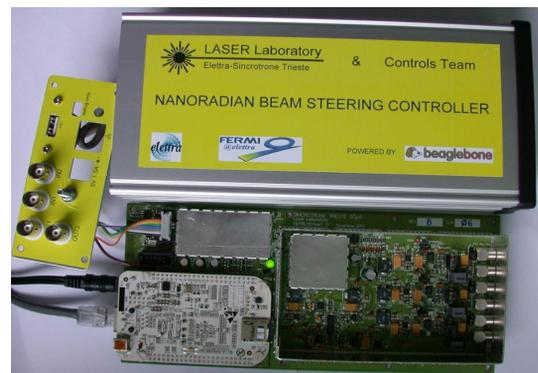
Figure 3: Tip-tilt Controller assembly.
