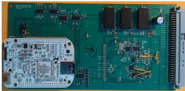
Figure 4: The NewPSC controller assembly with the BeagleBone and a prototype of the BBC.
