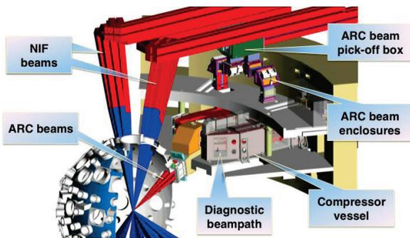
Figure 4: ARC system integration with NIF target area.
