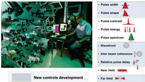
Figure 8: ARC laser diagnostic system overview
