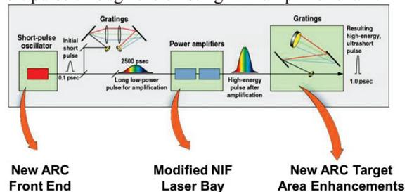
Figure 2: ARC short pulse generation and beamline propagation.
