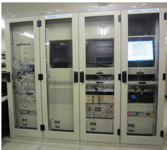
Figure 4: Digital LLRF system. FA-M3-based IOC is on the other side of the leftmost rack.
