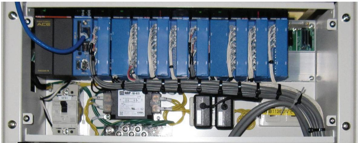
Figure 2: An example of FA-M3-based IOCs. The double-width black module is the power supply module. Next to its right is an F3RP61 CPU. All the other modulus in the figure are I/O modules.
