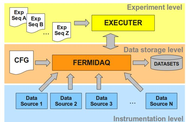
Figure 1: Block diagram of the FERMI experiment management system.
