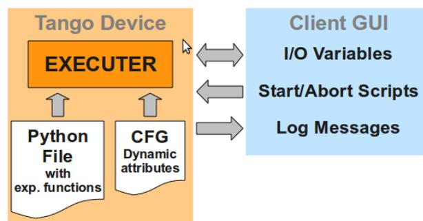
Figure 3: The EXECUTER Tango device can execute generic Python scripts, input and output variables can be defined in a XML configuration file.
