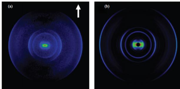
Figure 7: Example of a LDM VMI image. Photon energy 23.95 eV, circular polarization. Sample: He. (a) Raw data. The arrow indicates the direction of propagation of the light. (b) reconstructed image. [10]
