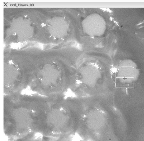
Figure 6: Sample scan at the EIS-TIMEX end-station: holes (50-100 micron diameter) produced by the pump-probe sequences in a Ge foil.
