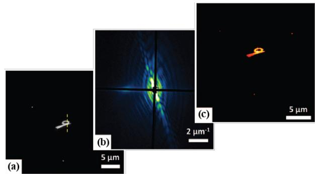
Figure 5: A DiProI CDI experiment. (a) SEM image of the sample. (b) Single shot diffraction pattern with 32.5 nm FEL pulse. (c) Phase retrieval reconstruction. [8]
