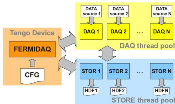
Figure 2: Structure of the multi thread FERMIDAQ Tango device.
