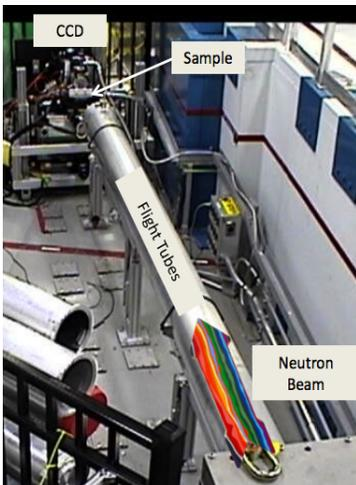
Figure 1: CG-1D neutron imaging beam line.
