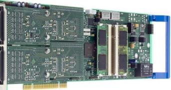
Based on a PCI 32 bit 125 MS/s digital I/O module from SPECTRUM with acquisition software running on a LINUX front-end
