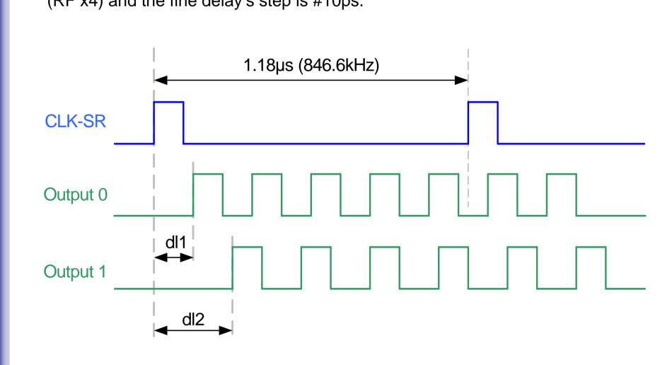
The two clocks high and low levels ratio can be adjusted by the user. This allows odd frequency division. For example for a RF / 17 division, the user can configure the output for 8 high levels and 9 low levels (8 + 9 = 17). Of course, he can also configure 1 high level and 16 low levels, or 16 high levels and 1 low level.
