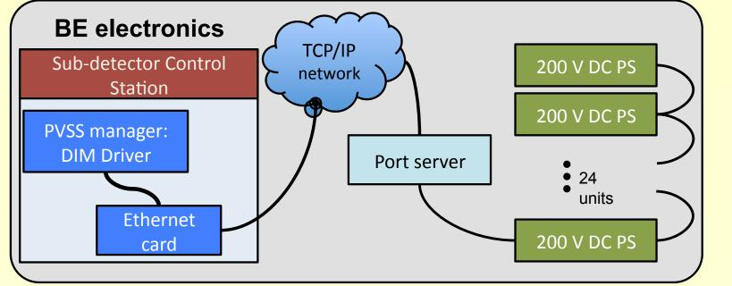
The Mod bus communication is established through the TCP/IP network, via the Port Server. The schematics of used Mod Bus readout chain is
