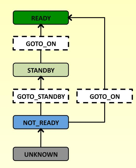
Figure on the right shows state diagram for the Tile Cal detector, where dashed lined boxes correspond to the implemented commands and the colored boxes represent allowed states. The arrows indicate allowed transitions between states.
