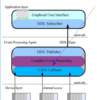
Event Processing Agent (EPA) aggregates, verifies, analyzes low-level DBPM data distributes and summarized results through DDS to the GUI. The EPA uses CAFE to establish a callback mechanism to EPICS:
