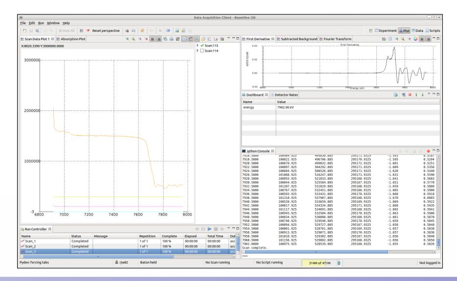
B18 was the first beamline at Diamond to use a GDA client based on the Eclipse RCP. Users define experimental parameters using graphical editors which persist the options in XML files. These feature rich editors give users a wide range of options to control the experiment. Validation of the XML files ensures that the options they choose are self-consistent and acceptable.
