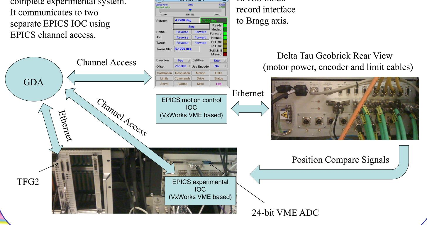
The Delta Tau has the ability to produce 'position compare' trigger pulses, based on the encoder position as the Bragg axis moves. These triggers are fed into the TFG2 VME card, which controls data acquisition.
