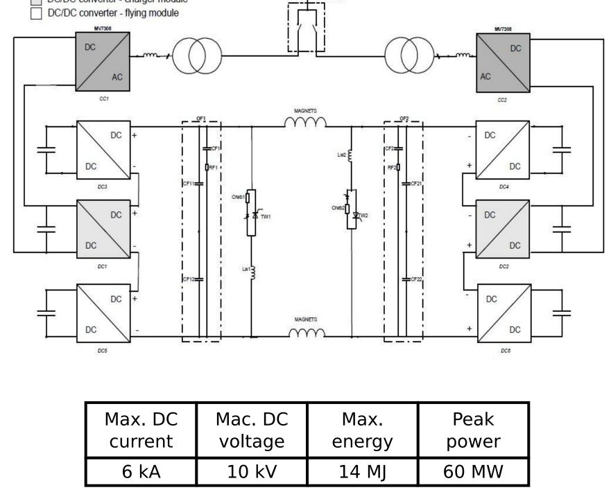
Three-level converters **Electrical network** AC/DC converters Capacitors banks DC/DC converters Load
