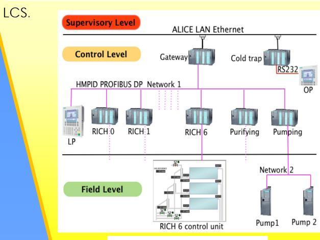
The hardware of the control layer consists of a network of Siemens S7-300 PLCs, one per control unit, reflecting the traditional Master-
