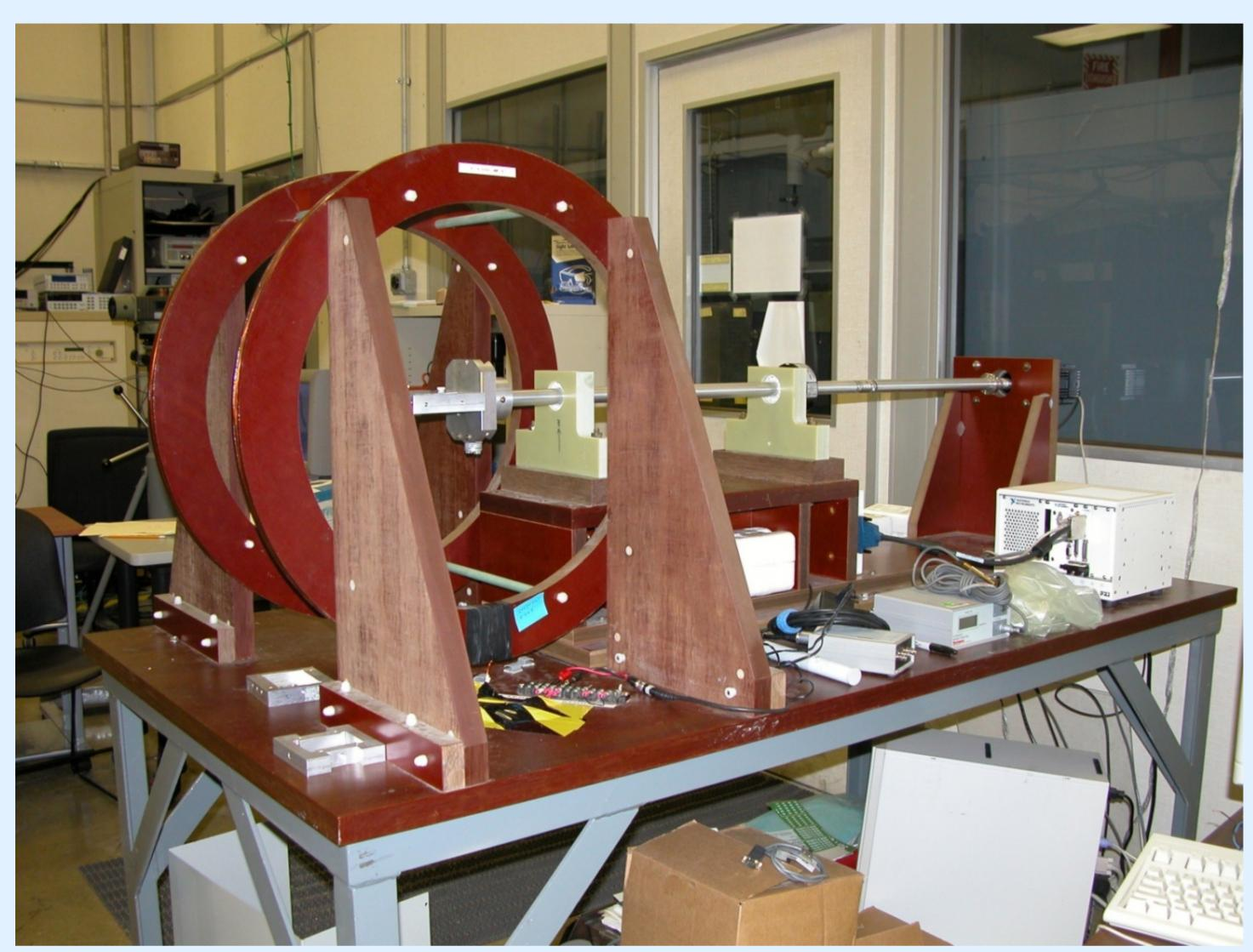
Figure 1. Helmholtz coil magnet measurement system.
