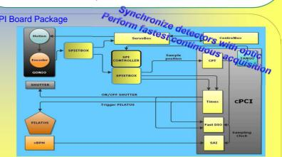
architecture implemented with SPICONTROLLER and SPIETBOX to make continous scan using Pilatus detector. It allows to:
