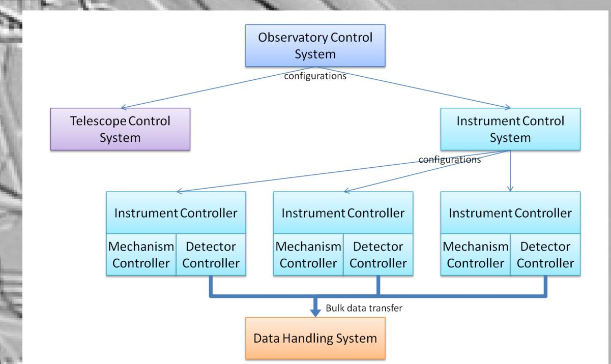
observation and must complete their data collection prior to the next telescope motion while other instruments may function in a complementary role – collecting data continuously until all the critical instruments are complete.
