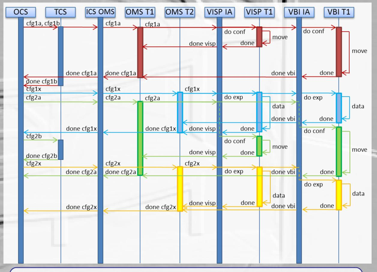
Sequencing of two steps in above script showing details of ICS control (OMS) threads and actions of two instruments (VISP and VBI).
