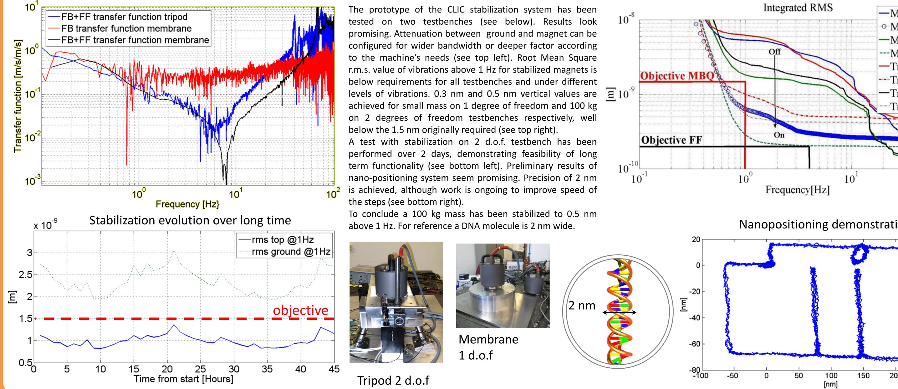
r.m.s vibration levels for different testbenches and conditions
