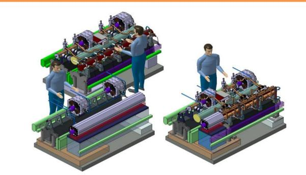
**Requirements stabilization:**  Transmissibility reduction >5 Bandwidth: 1-50 Hz • No resonances 50-100 Hz **Requirements nano positioning:** • Every 20 ms Steps of 20 nm • Precision +/- 1 nm **Additional requirements:**
