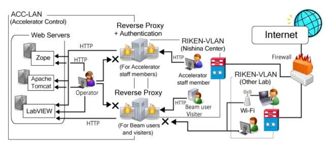
Figure 2: Network diagram in the web communication using reverse proxy servers between ACC-LAN used for RIBF control system and RIKEN-VLAN for office network.
