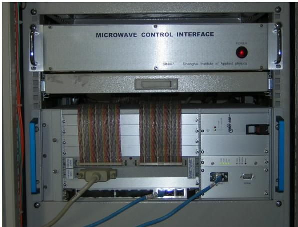
Figure 4: IOC controller and Interface.
