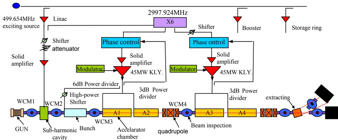
Figure 2: 150MeV Linac RF system layout.
