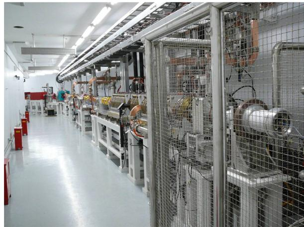
Figure 1: 150MeV Linac of SSRF.
