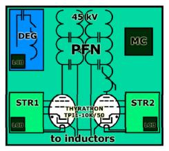
Figure 1: Modulator structure.
