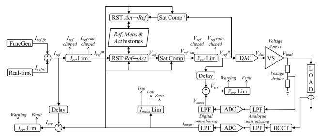
Figure 4: Overview of current regulation of an analogue voltage source.
