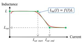
Figure 5: Magnet saturation model.
