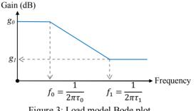
Figure 3: Load model Bode plot.
