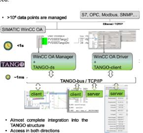
Figure 2: Schematic overview of the WinCC OA / TANGO interaction for beamline operation. The intrinsic time scale difference is managed by the developed WinCC OA manager and driver.
