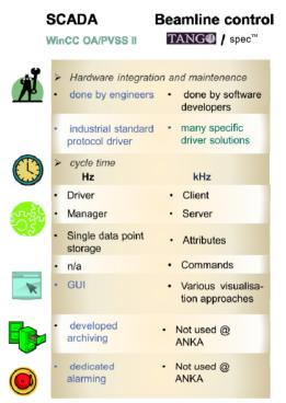
Figure 1: Comparison chart of basic features of WinCC OA and Tango based beamline control. Key benefits of the SCADA and TANGO used at ANKA are marked blue.
