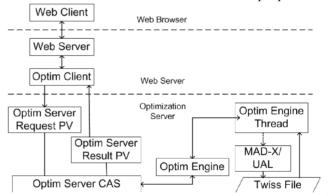
Figure 2: Example architecture of a middle-layer server.
