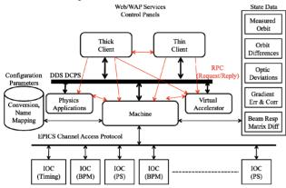
Figure 1: SOA for high-level applications over DDS.
