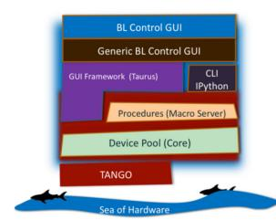
Figure 5: Conceptual design of Sardana.
