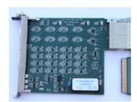
Figure 10: Fast/Slow ADC RTM (SLAC) mates to COTS Generic FPGA AMC (TEWS 651) for Klystron Interlocks Processing.
