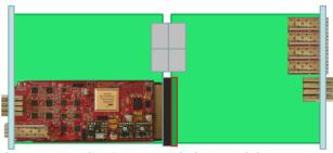
Figure 7: MTCA.4 Tx-Rx Timing Module Prototype (Stockholm University & DESY) and Double Wide Concept (in design, Stockholm).
