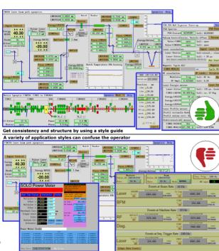
Figure 5: Use a style guide to make all operational tools similar to use. This increases the confidence of the operator in his tools and reduces the number of operator faults.
