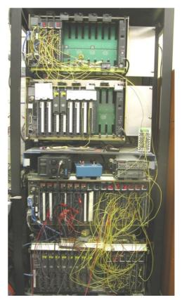
Figure 3: The mock-up system with wires simulating device feedback.
