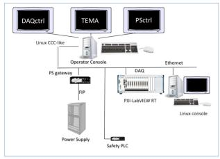
Figure 2: The control architecture.
