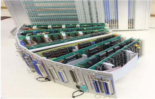
Figure 3: A variety of SABUS cards and a crate, most connectors compatible with CAMAC modules.
