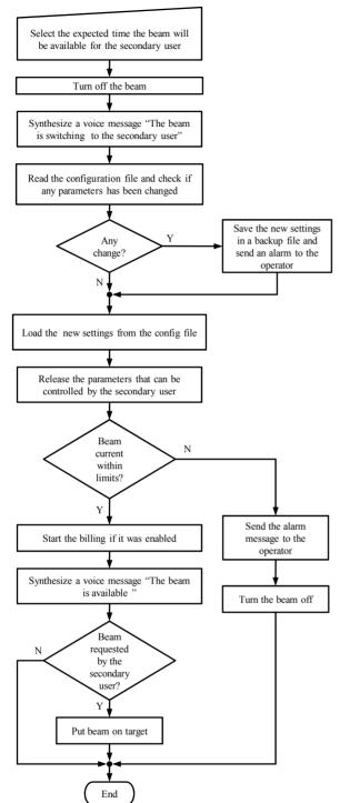
Figure 3: Beam switching from the therapy to the secondary user.
