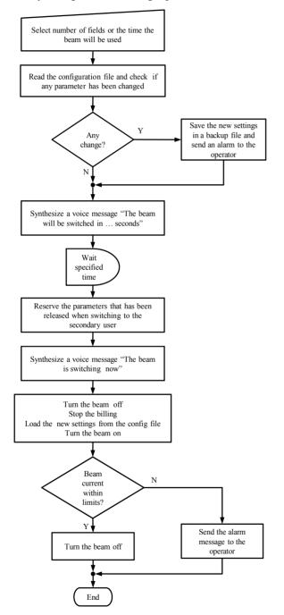
Figure 1: Beam switching from the secondary user to the therapy.
