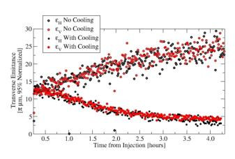
Figure 4: Horizontal and vertical emittances during two different physics stores. The open set of points show the normal increase due to IBS during a store. The solid points show decreasing emittances from transverse cooling. Measured using the RHIC IPM [21]
