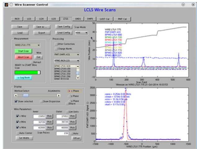
Figure 7: Snapshot of the wire scan graphical user interface showing x, y, and u wire scan signals during a single sweep (top right) and an individual wire scan plotted versus measured wire position (bottom right).
