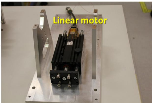
Figure 3: Linear motor slide assembly with magnetic shielding removed.
