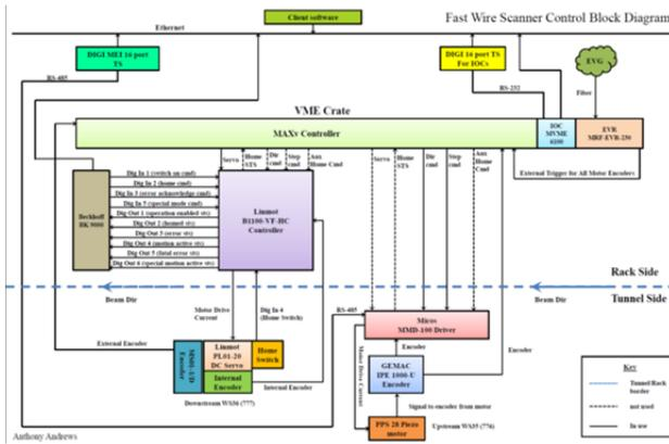
Figure 6: Block diagram of the wire scanner control system.
