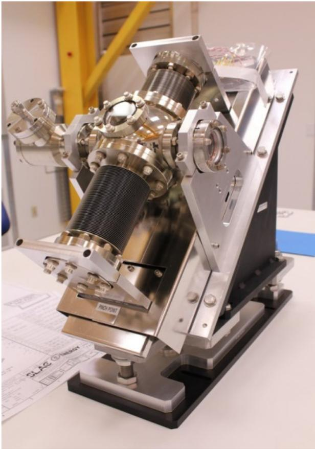
Figure 2: The wire scanner mounted on its 45° motion assembly.
