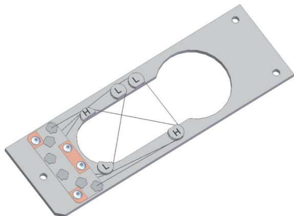
Figure 5: Wire card assembly showing how the x, y and u wires are mounted.
