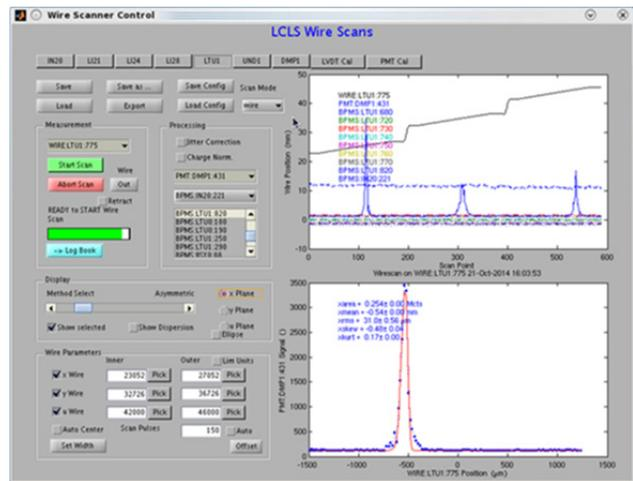
Figure 7: Snapshot of the wire scan graphical user interface showing x, y, and u wire scan signals during a single sweep (top right) and an individual wire scan plotted versus measured wire position (bottom right).
