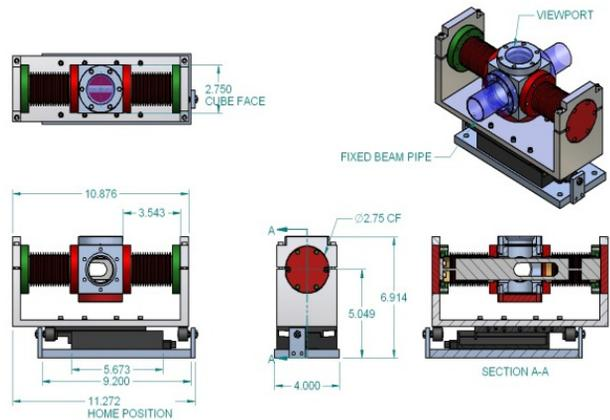
Figure 4: Mechanical sub-assemblies of the wire scanner.
