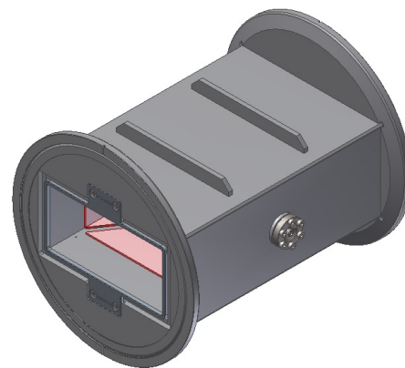
Figure 2: Linear-cut beam position monitor in KHIMA synchrotron.
