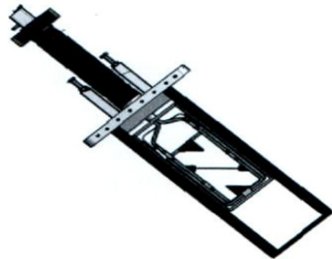
Figure 1: The Schematic view of the wire scanner.
