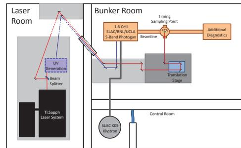
Figure 3: Simplified schematic of installation on the PEGASUS beamline.
