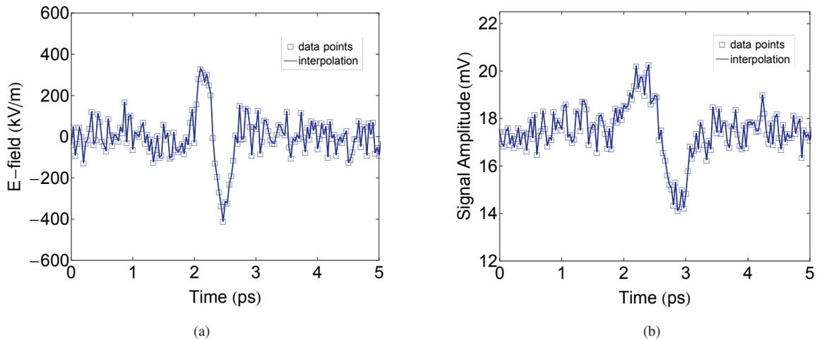
Figure 2: (a) EOS measurement and (b) PCA measurement of the single-cycle THz pulse generated through optical rectification on the bench-top set-up. The temporal profiles obtained by the two methods show comparable sensitivity to low THz power.
