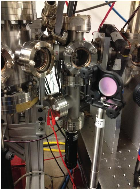
Figure 4: PCA mount with actuator installed in cross on PEGASUS beamline.
