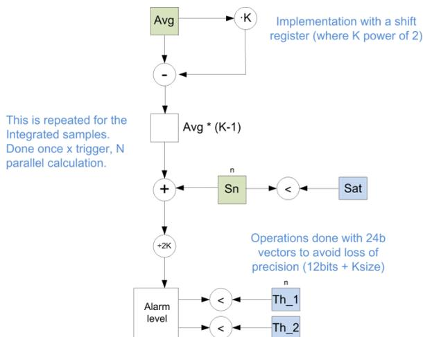
Figure 3: Flow diagram of the MPS algorithm.
