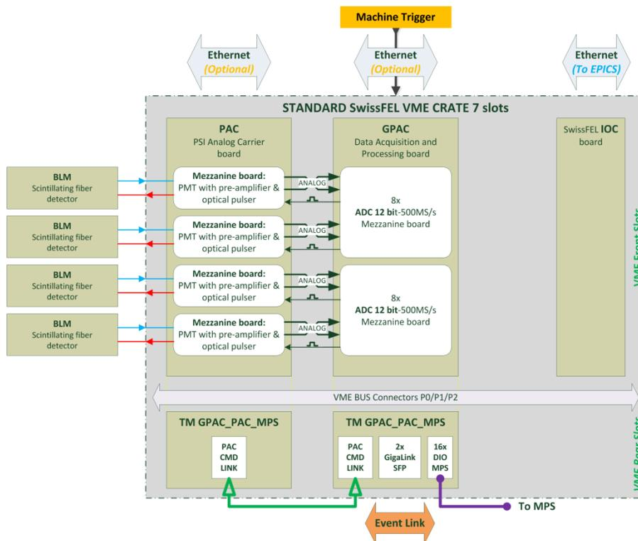
Figure 1: Sketch of the Beam Loss Monitor (BLM) electronic crate overview.
