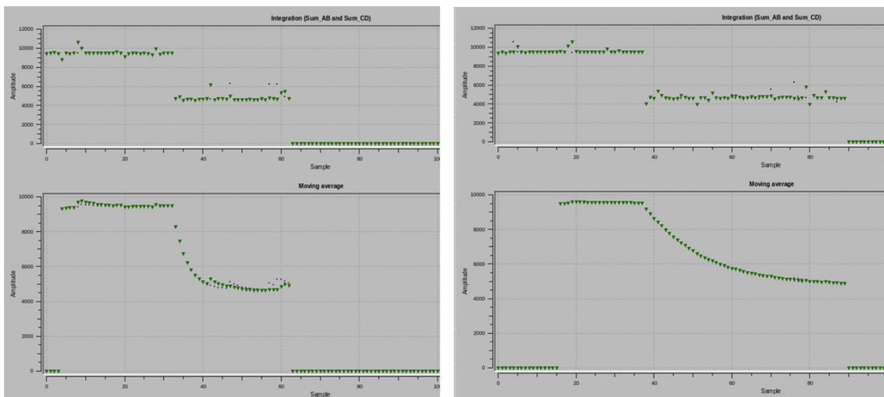
Figure 4: Results of the algorithm implementation shown for two values of K. The algorithm acts as a low pass filter (bottom plot) and removes noise from the shot-to-shot changes of the integrated signals (top plot). The filtered signal is used for triggering the MPS.
