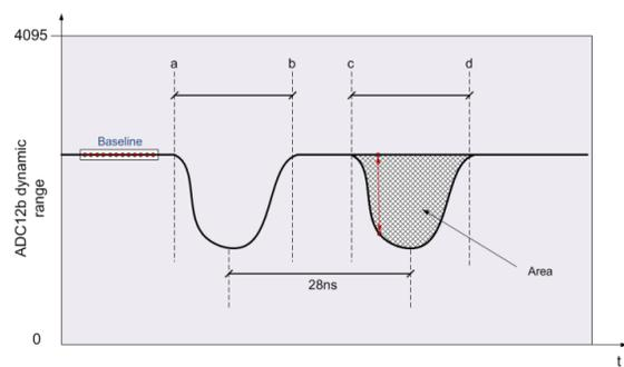
Figure 2: Schematic of the pulse integration.
