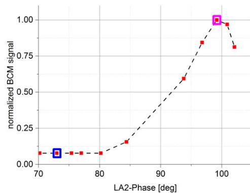
Figure 4: Normalized BCM signal for the SRF injector changing the bunch compression by adjusting the phase of the 2nd module.
