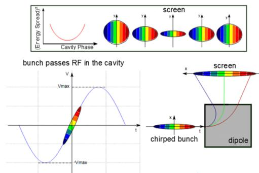
Figure 4: Illustration of phase scan technique [4].
