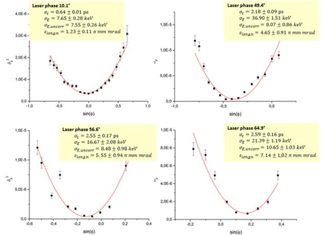
Figure 5: Energy spread measurement for four different laser phases with 19 MeV electron beam.
