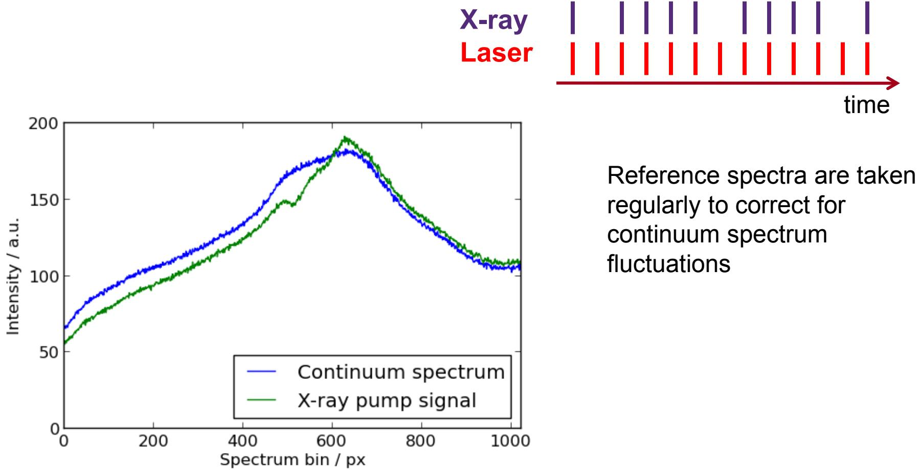
Reference spectra are taken regularly to correct for continuum spectrum fluctuations
