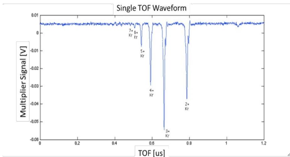
Typical time of flight ion charge spectrum for a single pulse using krypton as a target gas.
