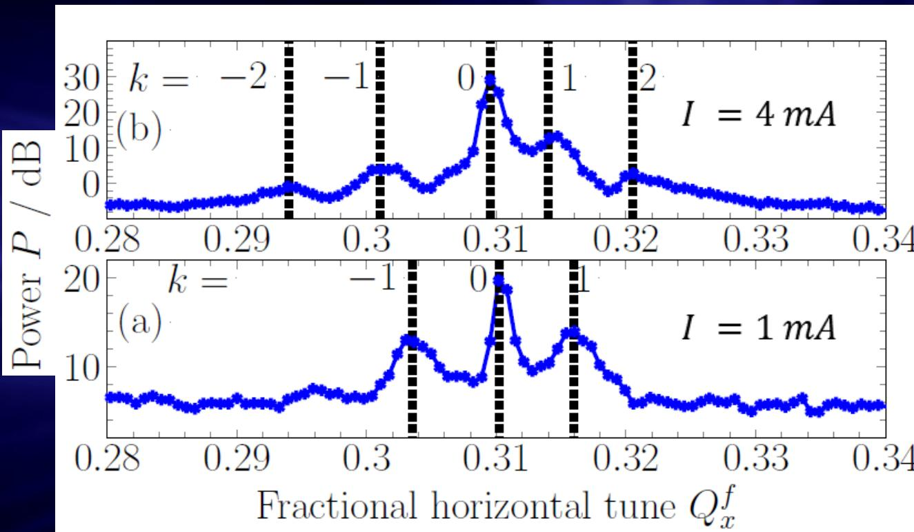
**Higher current:** The „global“ peak moves to the left. The symmetry of the spectrum is broken.
