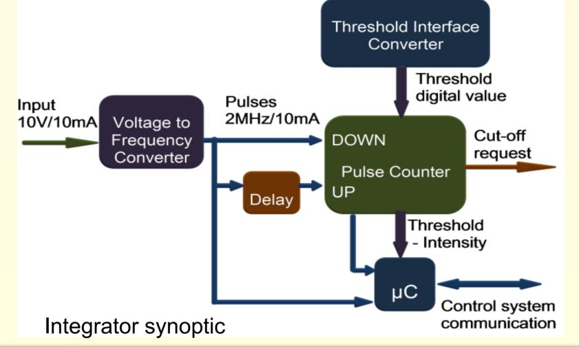
A microcontroller is used to perform the counting function and monitor the other thresholds with less reliability but more flexibility. The microcontroller manages the other functions like the communication between the electronics and the control system.
