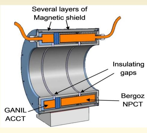
Transformer descriptions: DCCT: NPCT-175-C030-HR ACCT: Torus: Nanocristaline, Turn ratio: 300:1 Internal diameter: 184 mm, External diameter: 220 mm
