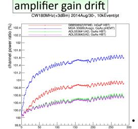
We measured amplifier gain drift of the BPF circuits in a thermostatic chamber (25±0.1 °C) for 286 hours (11.9 days).
