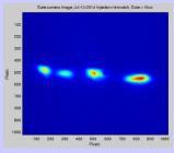
First several turns profile captured using gated camera after injection kicker
