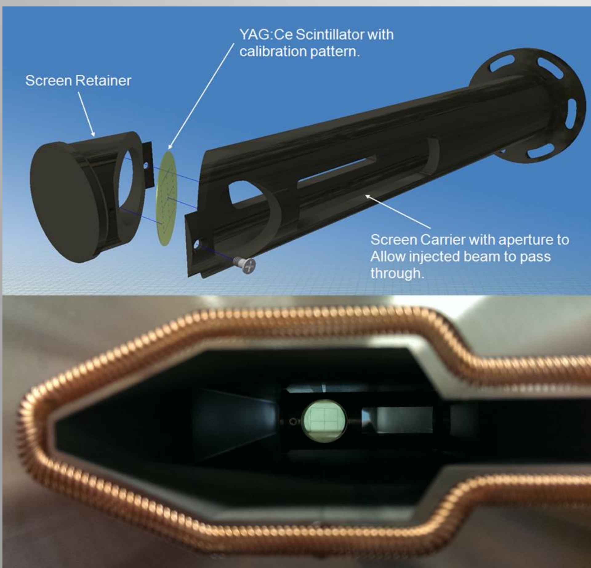
Figure 2: Screen in the parked position showing the RF spring. The HelicoFlex seal is also shown.
