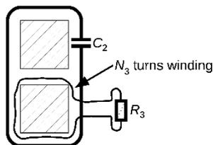
Figure 2: Cut through an ICT with an unwound core (top) and a read-out core with the read-out winding (bottom). The beam passes outside the box which encloses the cores.
