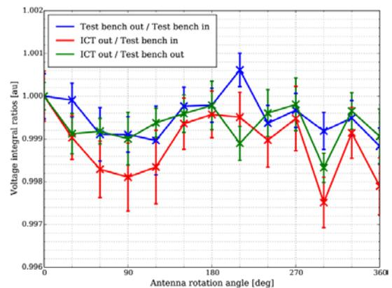
Figure 5: Measured beam position dependency.
