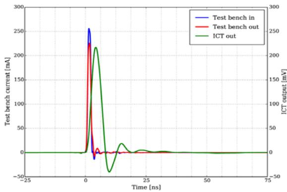
Figure 3: Time response of the ICT to an LHC bunch-like pulse.
