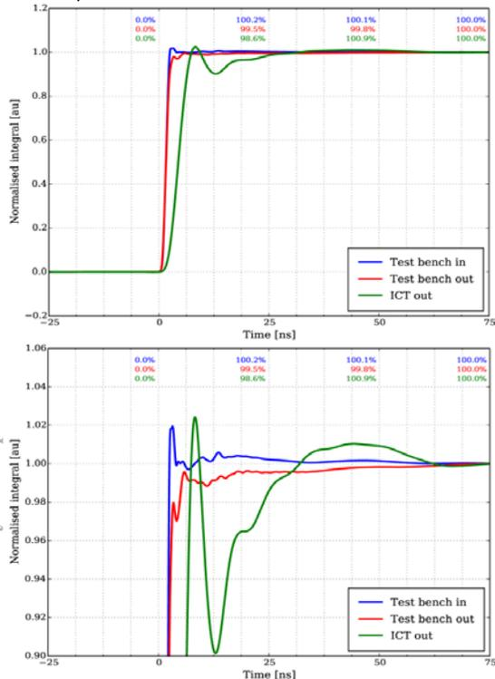
Figure 4: Normalised time integral of the ICT output pulse, with a zoom in to the region of interest in the lower plot.
