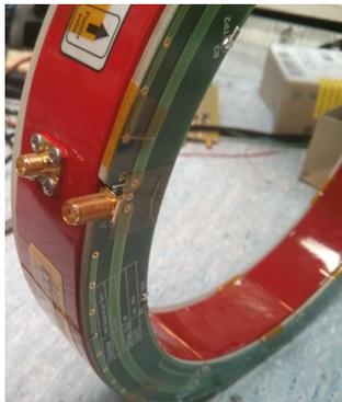
Figure 7: The installed calibration winding.
